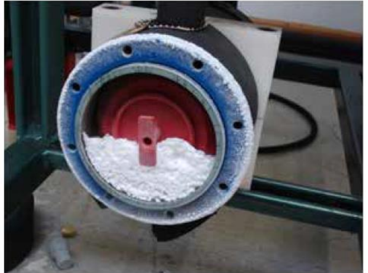
Figure 29. Example of dry ice formation in a drier
